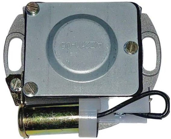
Photo 13 Assembled with gasket, cover, screws and washers
