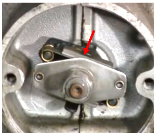
Photo 21 Points cam at rest. Note position of centrifugal weight (arrowed).
