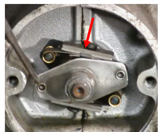
Photo 22 Points cam manually rotated 15° anti-clockwise (advanced). Note centrifugal weight position (arrowed).
